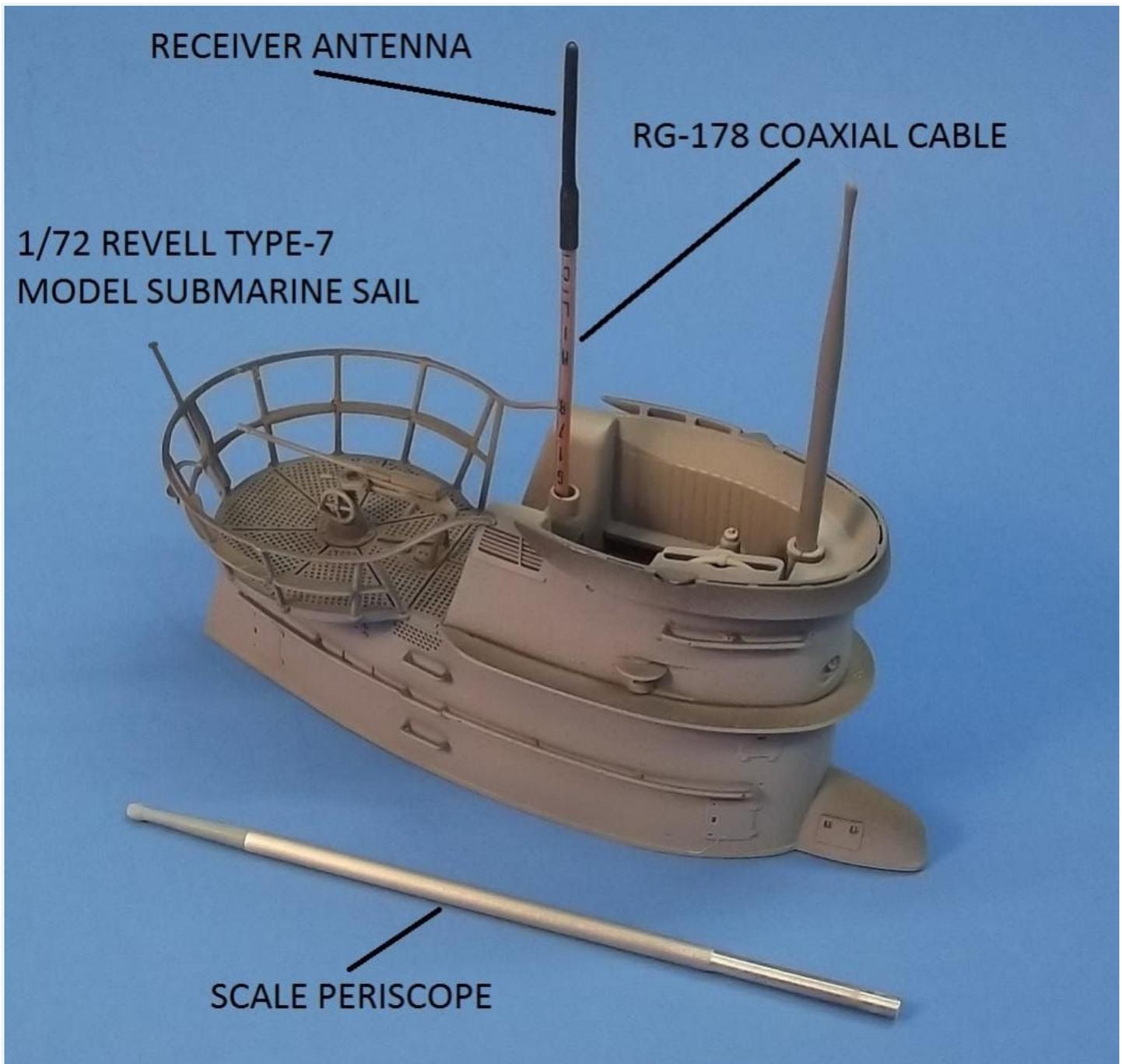
As illustrated here, you can employ a metal scope tube, to run the coaxial cable, but provide the upper portion (scope head) within which the antenna resides, as a plastic, RF transparent material. This arrangement puts the scope head above water -- and coincidentally, the antenna -- when operating the model submerged, at 'periscope depth'.
