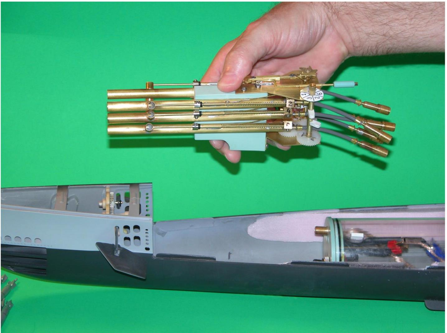
Mounting of the four tube nest at the stern of the GATO is done in a like manner. Of course there are variations of installation, the type and utility of the tube/nest installation you come up with is limited only by your imagination and craftsmanship.
