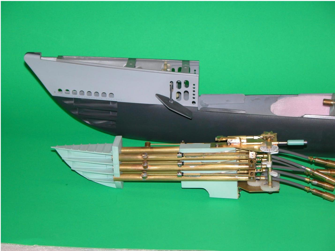
As you can see, things are a bit tight in the bow of the GATO with a complete set of launchers and the attached launcher trigger tripping mechanism.
