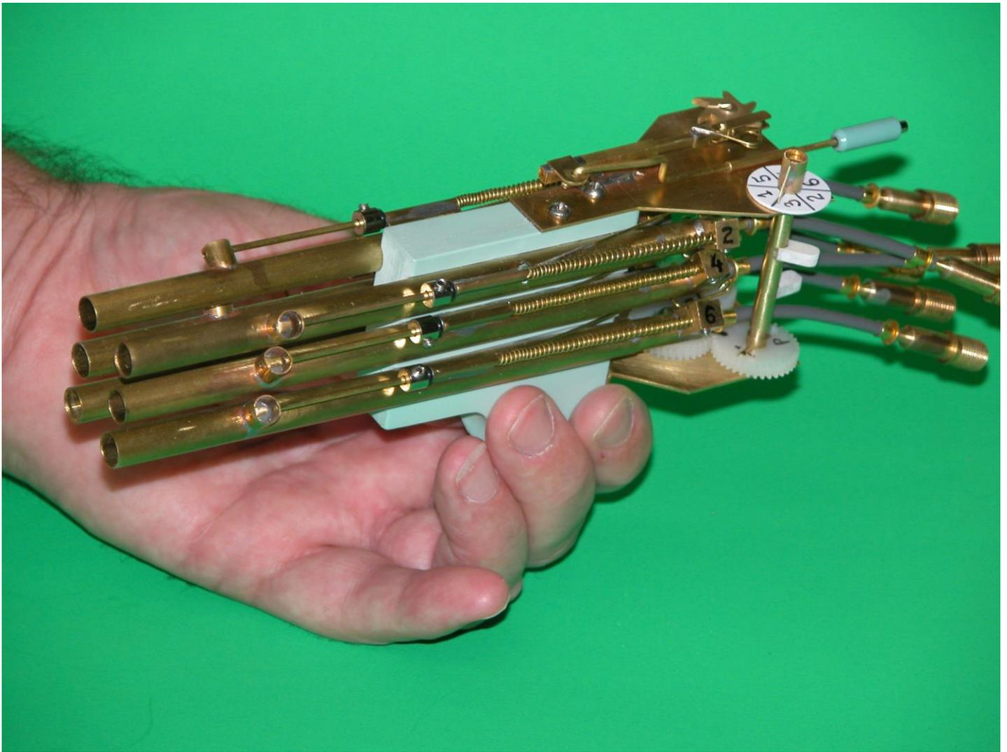
But, what if you wish to employ the Caswell-Merriman mechanical launchers in, say, a six-tube nest like what I've done for my GATO? In that case: you get creative! To help you out, I'll give you a little insight on how I designed, built, and installed a launcher trigger tripping mechanism onto the bow launcher nest of my 1/72 Revell GATO model submarine.
